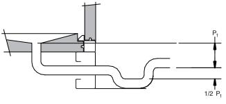
Fig. 20 — Condensate Drain Layout
